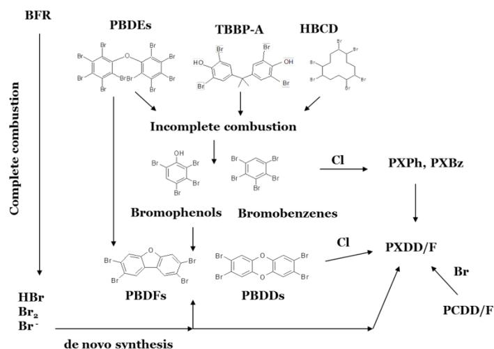
Figure 1: Pyrolysis and combustion of BFRs.
