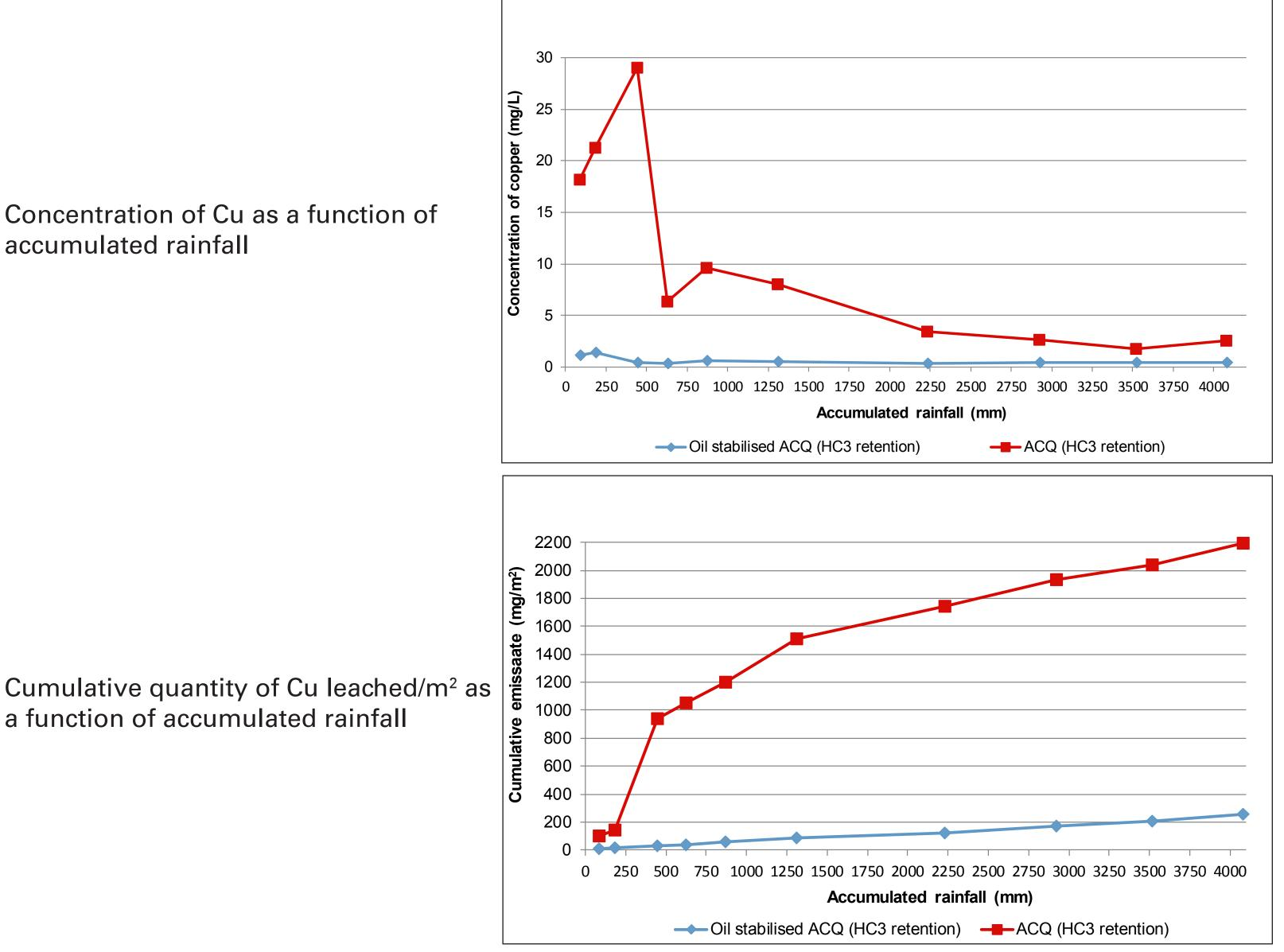
The total amount of copper emitted from the air-dried panels over 6 years was 4.4% of the amount in the wood after treatment. This result contrasts with a 'Tier 1' approach to calculating emission values for use in the BPD Scenarios, which could be used when no data are available, where 100% of the active substance is considered to leach immediately on exposure. In the case of wood preservatives this approach overestimates emission. Hense the risk to the environment.
