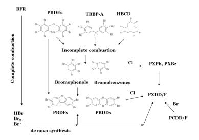
Figure 1: Pyrolysis and combustion of BFRs.
